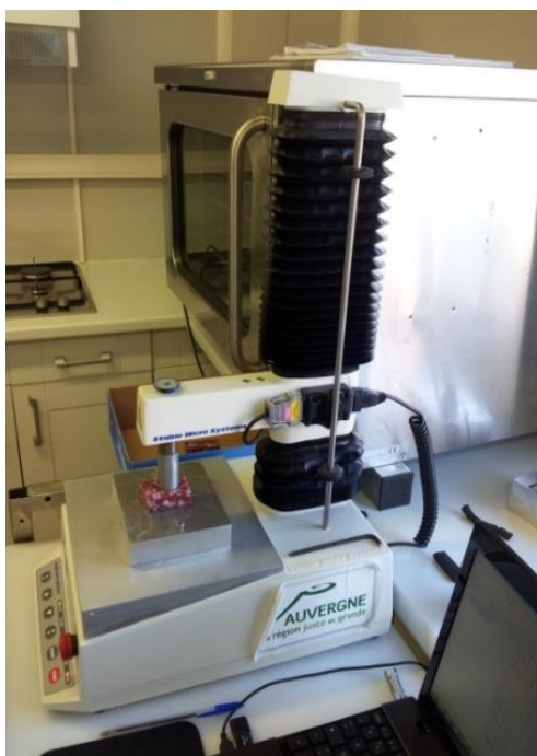
Figure 5. View of the texture profile analysis equipment used in this study to investigate the texture of all the DFS manufactured.
